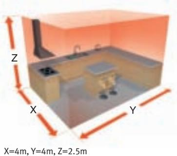
To decide which hood to choose, first calculate the volume of the room. This figure can be arrived at by multiplying room length x width x height. So a kitchen that is 4 x 4 x 2.5 metres has a volume of 40 m<sup>3</sup> (see diagram).
