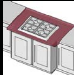
Step-out workstation with inset sink/hob
